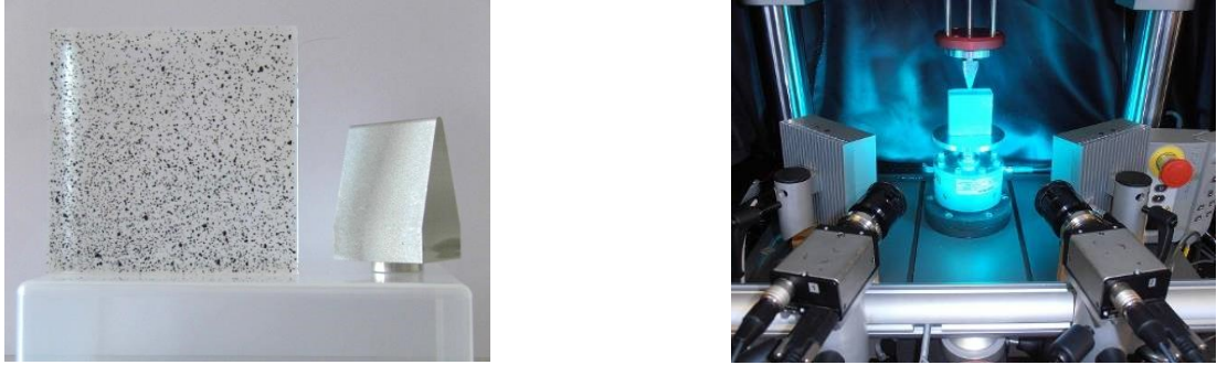
Figure 9: The specimen and experimental set up: rubber block (60x60x25mm) and the aluminium indenter with the 1.68mm radius tip and 73.45 degrees included angle (reproduced with permission from Tan et al [27]).
