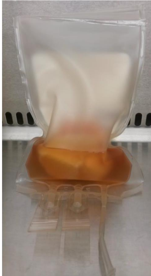
Figure 2.4.1. Hemi-condyle sealed inside a 1000 ml blood storage bag (R4R2022, Fenwal, London, UK) with tissue immersed in 100 ml Dulbecco's modified Eagle's Medium F12 Ham plus additions culture medium
