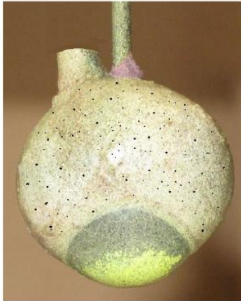
Figure 3.4. Intact porcine eye globe prepared for testing. Noted the proper alignment of the needle along with corneal apex.
