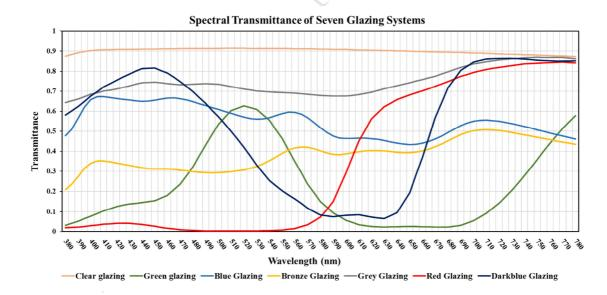
Figure 2. Spectral transmission of seven glazing systems studied in this office (China Academy of Building Research).
