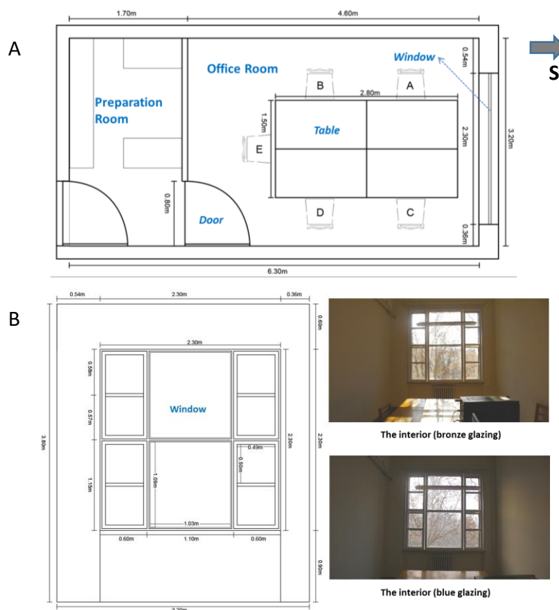
Figure 1. (A): Plan and dimensions of the office room; (B): Window configurations and dimensions (left), and interior views (bronze and blue glazing) (right).
