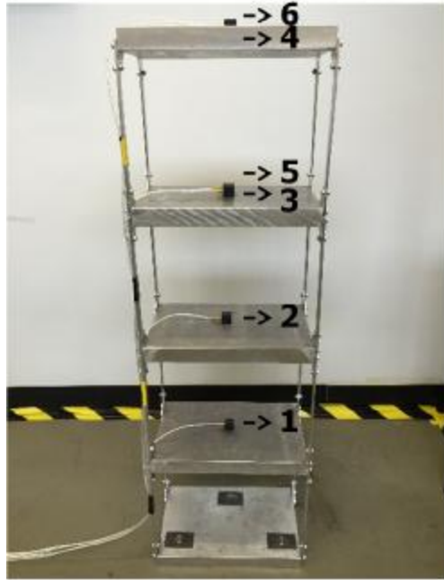
Figure 3. Four-storey Shear Frame
