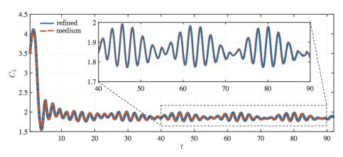
FIGURE 2. Time histories of lift coefficient obtained from two sets of meshes for the case of  $(\alpha, AR) = (22^{\circ}, 6).$
