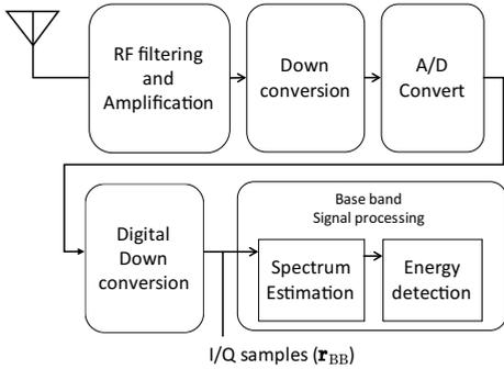
FIGURE 3: Block diagram of process in a sensor
