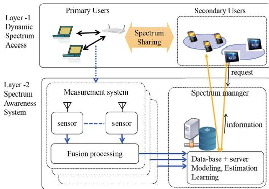
FIGURE 1: Concept of two-layered smart spectrum access (SSA)
