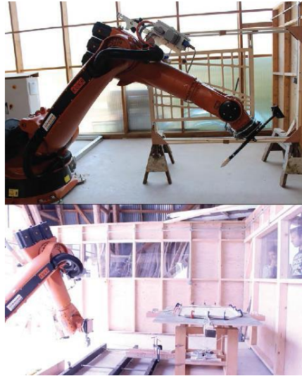
Figure 12: This shows the adhesive application and stretching operations, using the KUKA robotic arm
