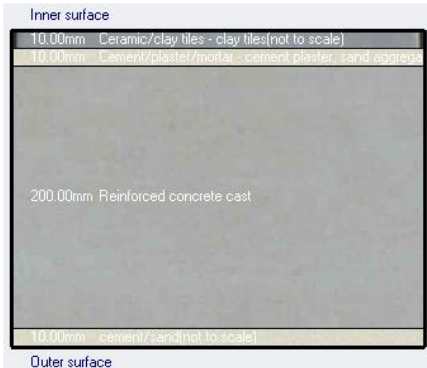
Figure C15 Internal floor concrete slab
