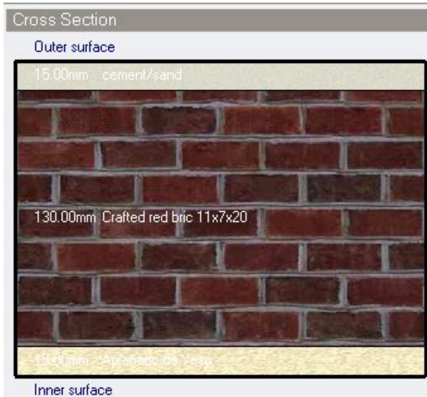
Figure C1 Red brick prototype external wall
