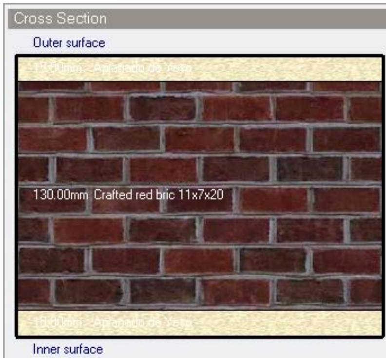
Figure C3 Red brick prototype internal partitions
