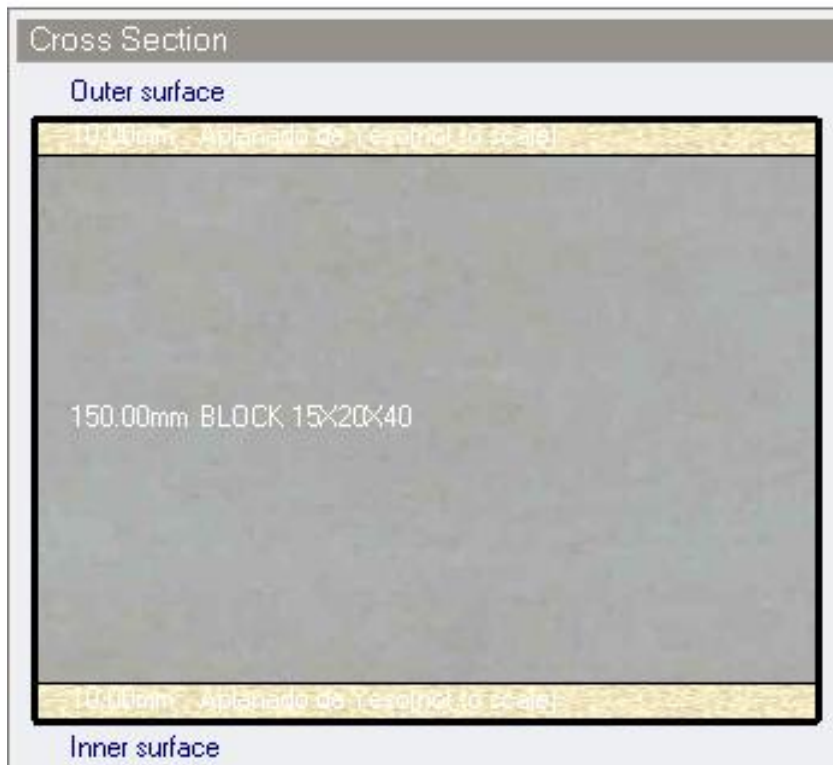
Figure C7 Hollow concrete block prototype internal partitions
