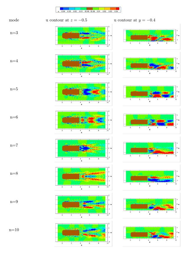
FIG. 14. Streamwise velocity contours of 3-D POD spatial modes 3 to 10 (from top to bottom); left) horizontal section at mid-height y = -0.5; right) vertical section at z = -0.4.
