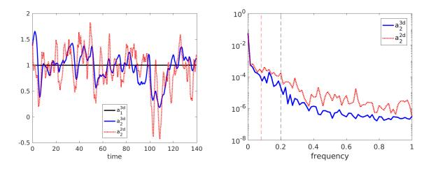
FIG. 12. Left) amplitudes of the first two POD modes; right) power spectral density of the quasisteady deviation mode  $|\hat{a}_2|^2$  - the red and black lines respectively correspond to the two frequencies 0.08 and 0.2.
