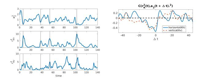
FIG. 16. Left) energy of POD modes corresponding to quasi-steady deviation  $a_2^2$ , spanwise  $(r_{Kh}^2 = a_3^2 + a_4^2)$  and vertical  $(r_{Kv}^2 = a_5^2 + a_6^2)$  vortex shedding intensities - vertical lines correspond to minima of  $a_2^2$ ; right) correlation coefficient between vortex shedding energy and quasi-steady deviation energy.
