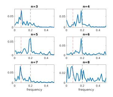
FIG. 8. 2-D POD amplitude power spectral density  $|\hat{a}_n|^2$  for modes 3 to 8 - the red and black dashed lines respectively correspond to the frequencies 0.08 and 0.2.
