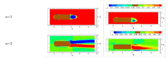
FIG. 11. Streamwise velocity contours of 3-D POD modes 1 (top row) and 2 (bottom row); left) horizontal section at mid-height z = -0.5; right) vertical section at y = -0.4.
