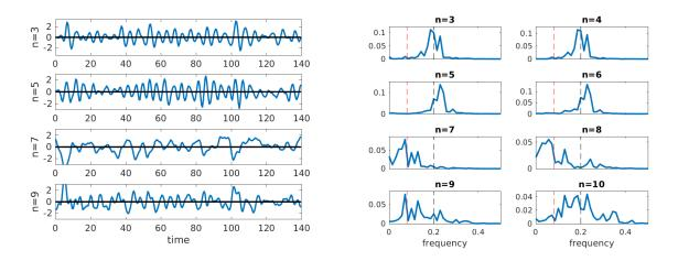
FIG. 15. Left) amplitudes of the modes  $a_n$ , n=3, 5, 7, 9; right) power spectral density of the 3-D POD mode amplitudes in the simulation  $|\hat{a}_n|^2$  - the red and black lines respectively correspond to the two frequencies 0.08 and 0.2.
