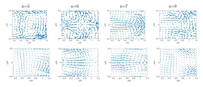
FIG. 7. 2-D wake POD modes 5 to 8; top row: simulation; bottom row: experiment.
