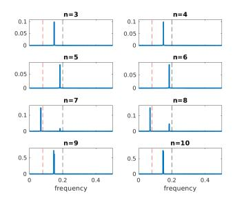
FIG. 18. Power spectral density of the 3-D POD mode amplitudes 3 to 10  $|\hat{a}_n^{3D,M_0}|^2$  in the simplified model - the red and black lines respectively correspond to the two frequencies 0.08 and 0.2.
