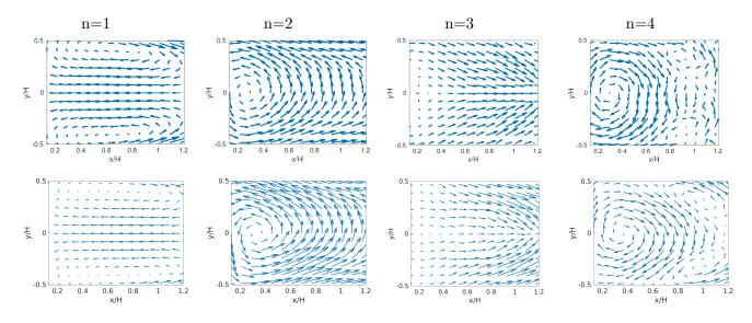
FIG. 4. 2-D wake POD modes 1 to 4; top row: simulation; bottom row: experiment.
