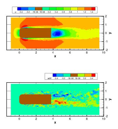
FIG. 10. Streamwise velocity contours on mid-height plane z = -0.5; top : projection of an instantaneous field  $\underline{u}$  onto the first ten modes  $u_{recons} = \sum_{n=1}^{10} a_n(t) \underline{\phi}(\underline{x})$  where  $a_n = \int \underline{u}(\underline{x}, t) \underline{\phi}(\underline{x}) d\underline{x}$ .; bottom: difference field  $|u - u_{recons}|$ .
