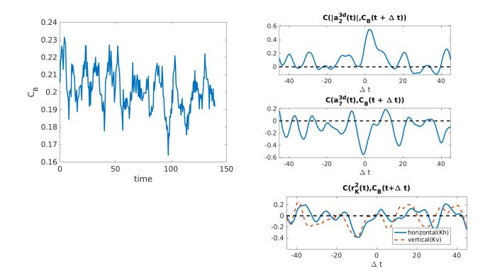
FIG. 17. Left) base suction coefficient  $C_B = -C_p$  obtained by integrating the pressure over the rear of the body; right) correlation between the base suction coefficient and the POD amplitudes corresponding to the steady deviation ( $a_2$ , top), wake pumping mode ( $a_7$ , middle) and vortex shedding modes ( $r_{Kh,v}^2$ , bottom).
