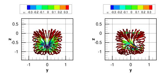
FIG. 13. Streamlines of the field viewed from downstream left) mode 1  $\sqrt{\lambda_1} \underline{\phi}_1$ ; right) combination of mode 1 and mode 2  $\sqrt{\lambda_1} \underline{\phi}_1 + \sqrt{\lambda_2} \underline{\phi}_2$ .
