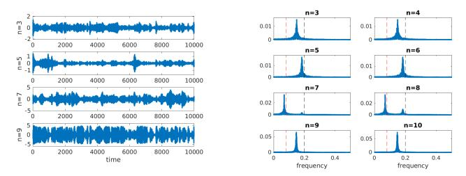
FIG. 20. Left) amplitudes of 3-D POD amplitudes of modes 3, 5, 7 and 9 in the model; right) power spectral density of POD amplitudes in the model  $|\hat{a}_n^{3d,M}|^2$  - the red and black lines respectively correspond to the two frequencies 0.08 and 0.2.
