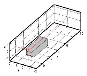
FIG. 1. Numerical configuration. The Ahmed body and the recirculation zone behind it are idenfied by a surface of zero streamwise velocity. The streamwise, spanwise and wall-normal positions are referred to as x, y, z. The length, width and height of the body are respectively L, W and H. The origin of the axes is taken at the top and foremost position of the Ahmed body in the vertical symmetry plane.
