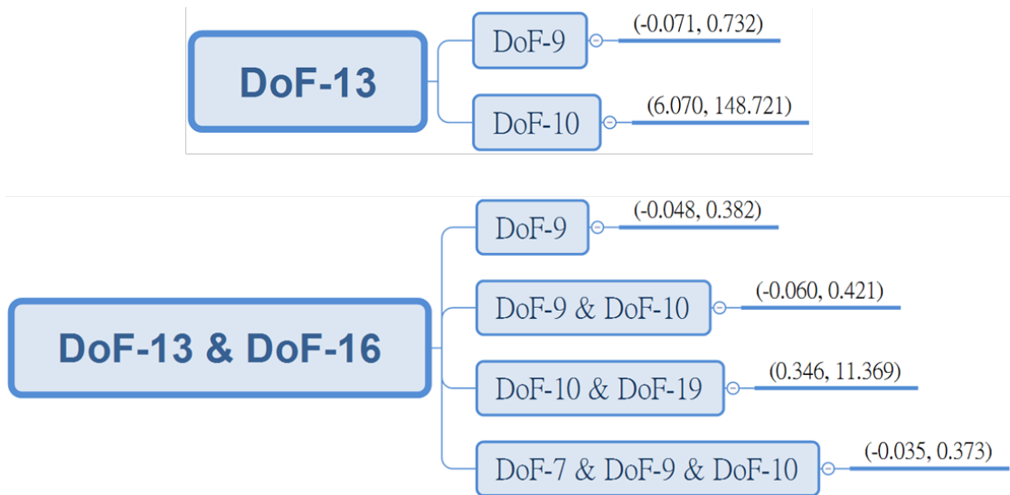
Figure 6. 9. Different combinations of excitations and responses. The blocks, from left to right, represent the DoFs for excitation, DoFs for measured responses, and the mean and variance of the corresponding result.
