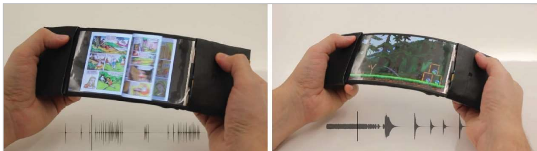
Figure 54. ReFlex bending to flip pages (left) and to play a game (right) (Human Media Lab, 2016)
