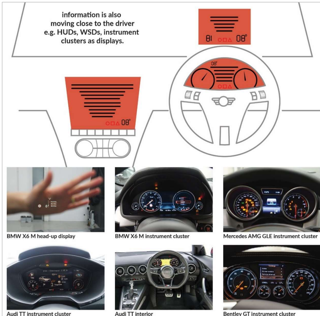
Figure 17. Information moving close to the driver, with behind-wheel displays becoming more content-driven
