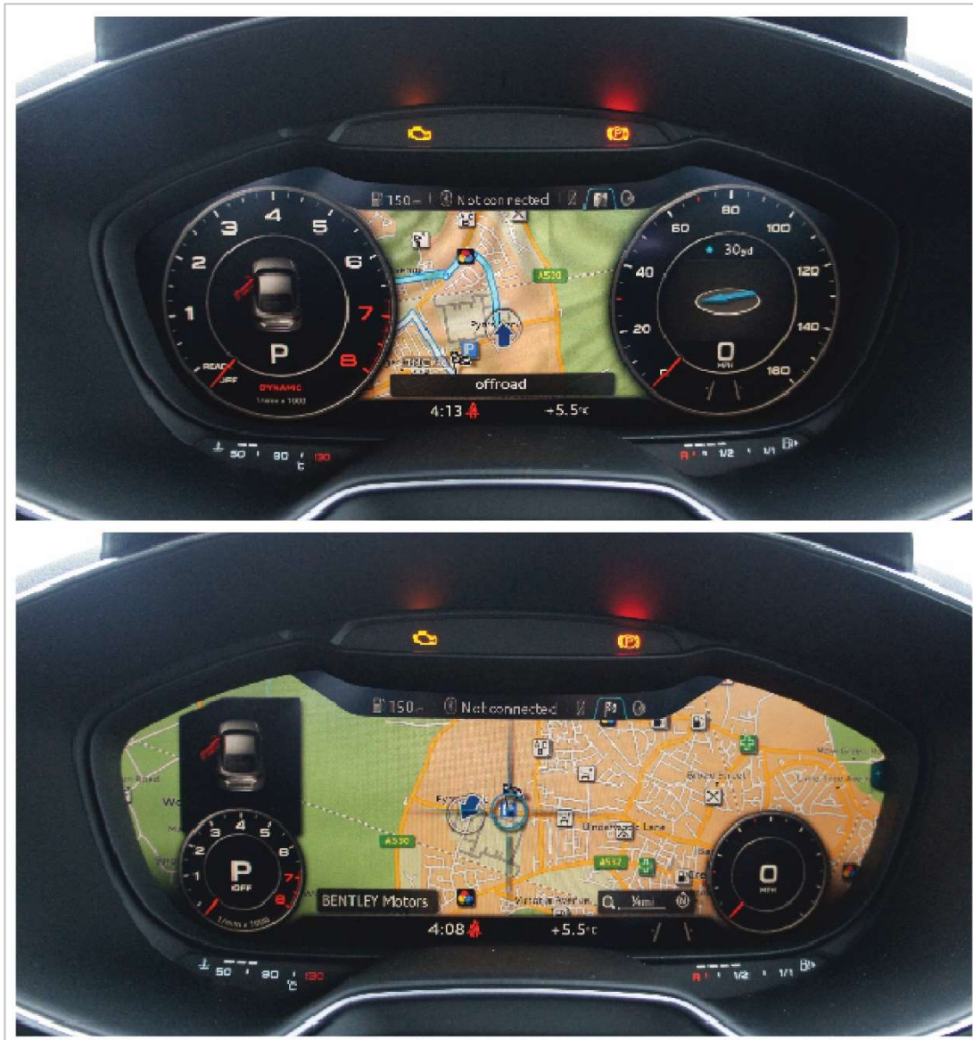
Figure 36. Reconfigurability of Audi TT LCD instrument cluster
