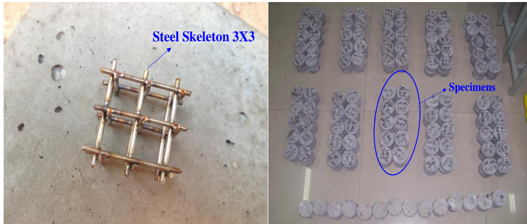
Figure 4.10 Steel skeleton (left) and the specimens (right).
