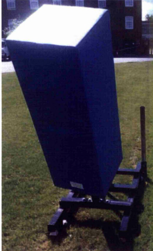
Figure 7.1 The bespoke 'contact sled' designed for simulating contact
