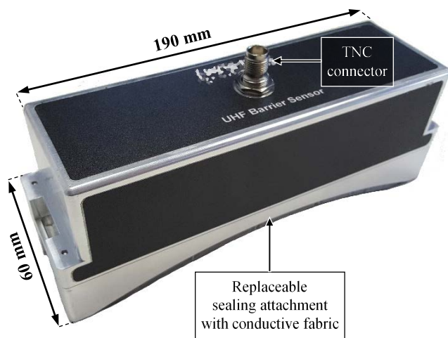
Fig. 8. UHF Barrier sensor, showing main components and dimensions. The replaceable sealing attachment allows the sensor to be installed on HV equipment of different sizes.
