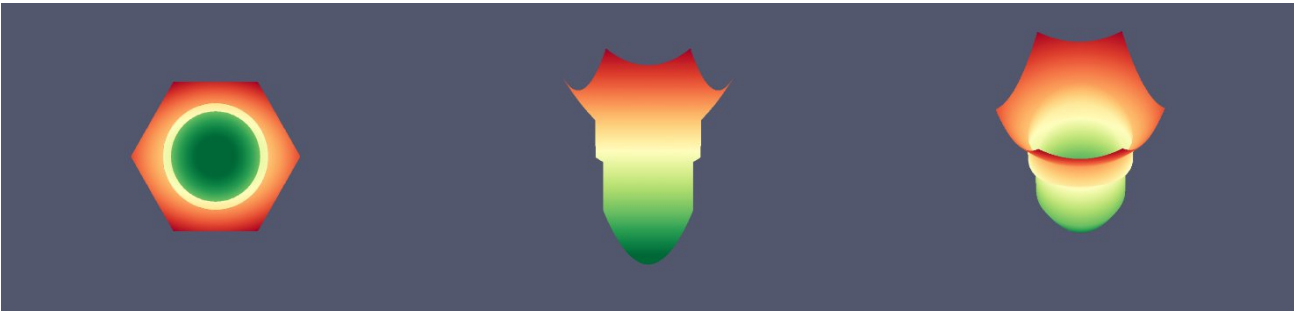
Figure 15. Plane (left), axial (middle) and 3D (right) views of the neutron flux distribution within hexagonal fuel cell calculated with transport solver ( P_2 approximation)
