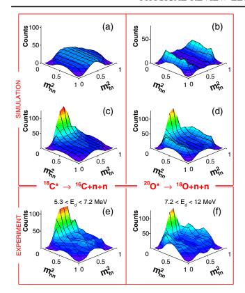
FIG. 2. Dalitz plots of fragment + n + n decays (fragment-n vs n-n normalized squared invariant masses). The three left panels correspond to  $^{16}C + n + n$ ; the right panels to  $^{18}O + n + n$ . The four upper panels represent simulations of (a) phase space, (b) sequential decay through a fragment-n resonance, (c) direct decay with n-n FSI, and (d) a combination of the latter two. The lower panels (e,f) correspond to the experimental data for the decay energies noted.
