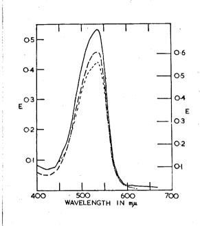
Absorption spectrum of zinc dithizonate in carbon tetrachloride (0.5 ug. Zn/ml.)
