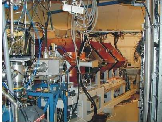
Figure 3.9: The Recoil Ion Transport Unit RITU in position at the University of Jyväskylä.
