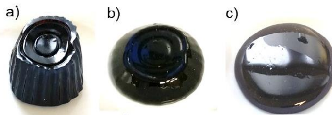
Figure 1.2.1 Images of sulfur-limonene copolymer a) after removal from mould, b) 2 hours at room temperature and c) 24 hours at room temperature
