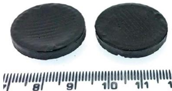
Figure 3.4.1 Image of moulded linear sulfur copolymers (S-FAR and S-MYR), with a centimetre ruler for scale
