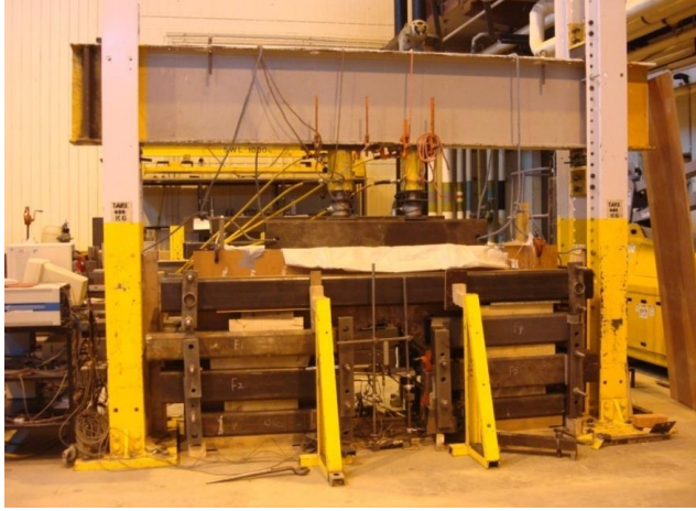
FIG 3. Loading system installation for uniform load
