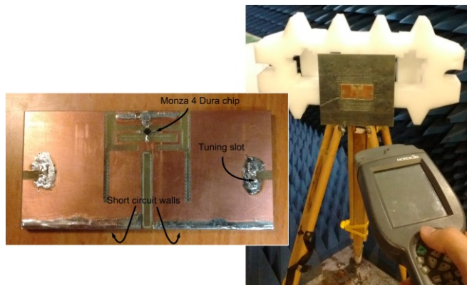
Fig. 12. Prototype of the proposed design and measurement setup in anechoic chamber.
