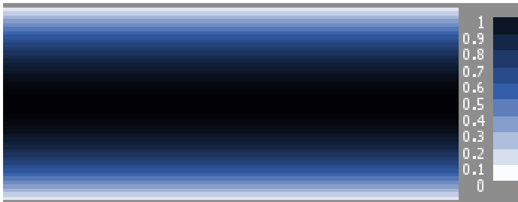
Figure 4.4 Normalised velocity flow profile from the Poiseuille flow NetLogo model with reflective boundaries and a force applied via gravity
