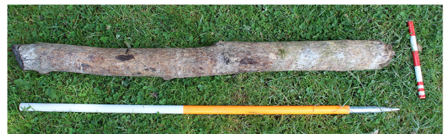
Fig. 15 Timber removed from original Cookhouse reconstructed wall, with part below ground missing
