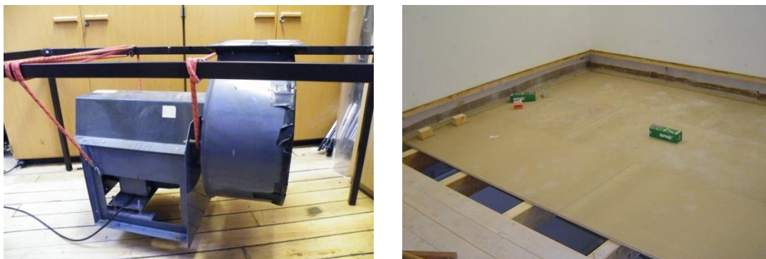
Fig. 14 - Fan, resiliently suspended in laboratory; timber joist chipboard floor under construction.
