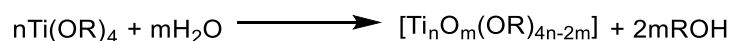
Scheme 6.1.2.1. Reaction pathway of TTIP and H 2 O to form a titanium oxo-cluster
