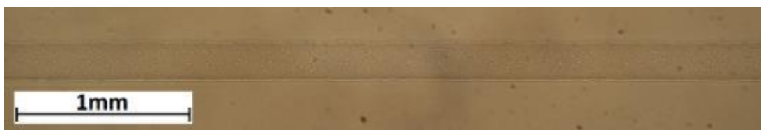
Figure 6.3.1.1 Printed track using ink 6.3.1 at 6 \text{ mm s}^{-1} print speed and 0.1 \text{ mm} step size on a glass substrate
