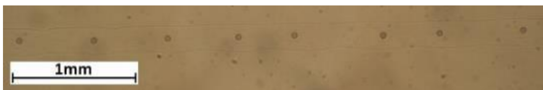
Figure 6.3.1.3 Printed track using ink 6.3.2 at 10 \text{ mm s}^{-1} print speed and 0.1 \text{ mm} step size on a glass substrate
