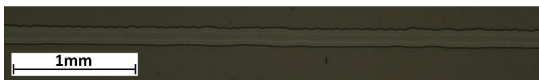
Figure 4.3.2.1 Printed track using ink 4.3.2 at 10 mm s -1 print speed and 0.1 mm step size on a glass substrate
