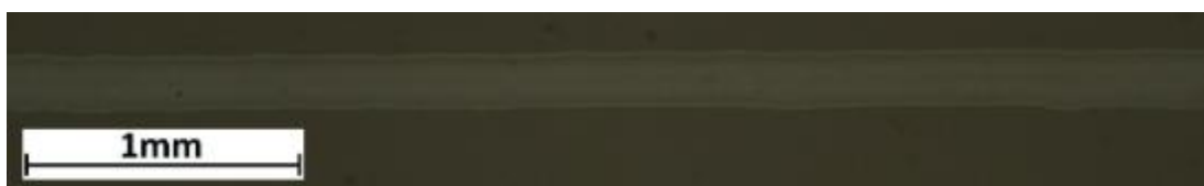
Figure 7.2.1.7 Printed track using ink 7.2.3 at 6 mm s -1 print speed and 0.2 mm step size on a glass substrate at 60°C stage temperature
