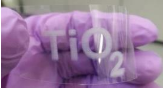
Figure 5.3.7.3 Printed 3 pass 'TiO 2 ' using ink 5.3.2 at optimised print conditions on a PET substrate
