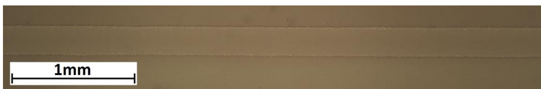
Figure 4.3.1.1 Printed track using ink 4.3.1.a at 10 mm s -1 print speed and 0.1 mm step size on a glass substrate
