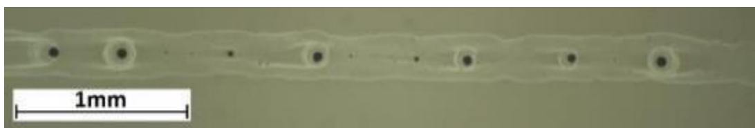
Figure 6.3.2.1 Printed track using ink 6.3.5 at 10 mm s -1 print speed and 0.1 mm step size on a glass substrate
