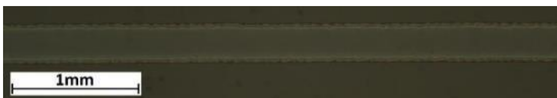
Figure 7.2.2.1 Printed track using ink 7.2.4 at 6 mm s -1 print speed and 0.2 mm step size on a glass substrate at 60°C stage temperature
