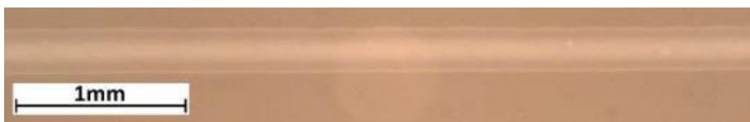
Figure 7.2.1.4 Printed track using ink 7.2.2 at 6 mm s -1 print speed and 0.2 mm step size on a glass substrate at 60°C stage temperature
