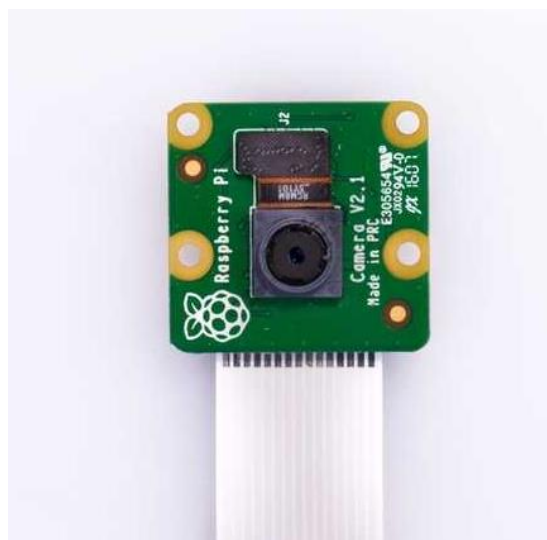
Figure 3-7: Raspberry Pi camera module version 2 used as the source for camera modelling parameters [112]
