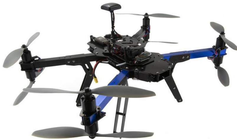
Figure 3-2: 3DR X8 co-axial quadcopter RUAS platform operated by the University of Liverpool [101]
