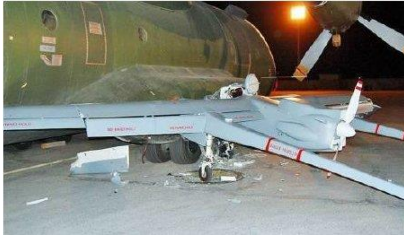
Figure 1-3: The aftermath of a collision between an RQ-2 Pioneer aircraft and a C-130 Hercules [24]
