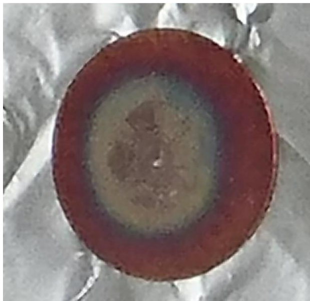
Figure 59: Cu-electrode of Li|SE|Cu cell after plating experiment, showing evidence for lithium metal plating. From Chem. Mater. 2018 , 30, 7183-7200. Reprinted with permission from ACS Publications.
