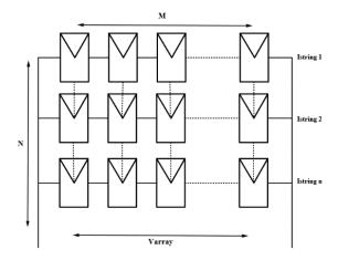
**Figure 8.** A series-parallel (SP) PV array involving  $N \times M$  (number of parallel-connected strings  $\times$  number of series-connected PV modules).
