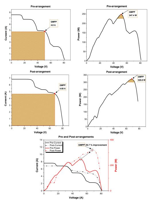
Figure 11. The output of the Array (pre-post rearrangements) for case 1.
