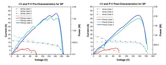
**Figure 14.** The outputs of a PV Arrays pre and post reconfigurations.
