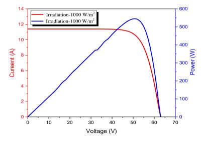
**Figure 5.** Simulation responses: *I-V* curve and *P-V* curve (at standard test conditions) for good quality modules of Solarex MSX60 connected in series.
