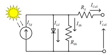
Figure 3. The equivalent of a single diode circuit of PV cell.
