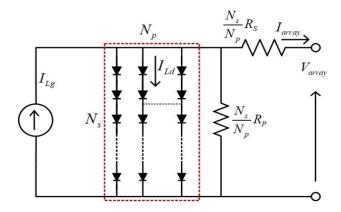
Figure 4. Equivalent circuit of PV array.
