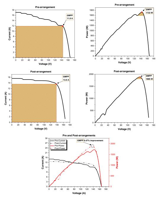
Figure 12. The output of the Array (pre-post rearrangements) for case 2.
