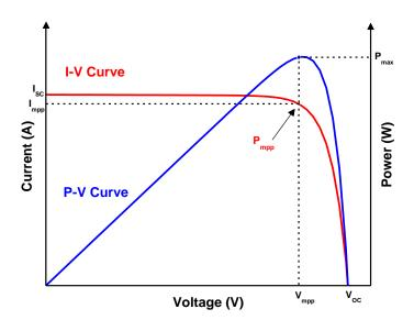
Figure 2. PV cell curve characteristics.
