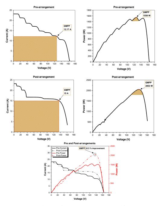
$\textbf{Figure 13.} \ \ \text{The output of a PV array (pre-post rearrangements) for case 3.}$
