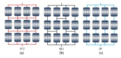
**Figure 1.** The fundamental formats of photovoltaic (PV) array linking are (a) total cross-tied (TCT), (b) bridge-link interconnection (BLI) and (c) series-parallel (SP).
