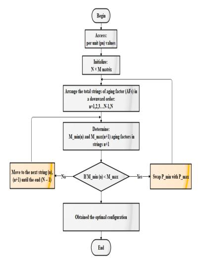
Figure 10. Flowchart of PV reconfiguration algorithm process.
