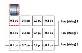
**Figure 9.** A  $3 \times 4$  PV array SP configuration with non-uniform aging.
