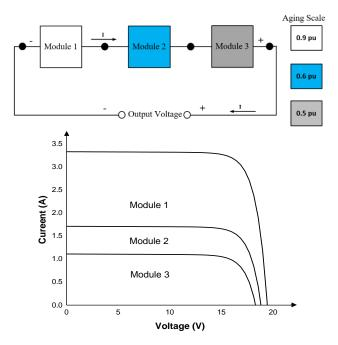
Figure 6. Series-connection of PV modules.
