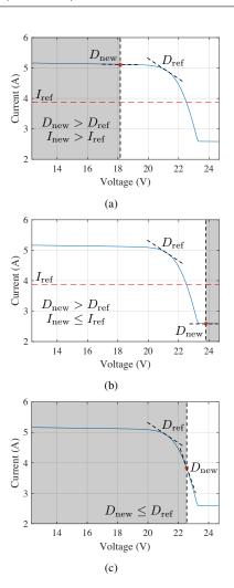
**FIGURE 4.** The judging criterion for three different cases: (a) case 1:  $D_{\text{new}} > D_{\text{ref}}, I_{\text{new}} > I_{\text{ref}}$ ; (b) case 2:  $D_{\text{new}} > D_{\text{ref}}, I_{\text{new}} \leq I_{\text{ref}}$ ; (c) case 3:  $D_{\text{new}} \leq D_{\text{ref}}$ .
