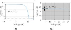
FIGURE 3. Initial selection rule for the Tabu List: (a) overall I-V curve; (b) region A; (c) region B.
