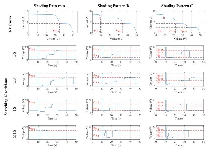
**FIGURE 6.** Comparison in the tracking traces from different searching algorithms under varied shading patterns (shading pattern A:  $\{500,1000,1000,1000\}$ W/m<sup>2</sup>,  $25^{\circ}$ C; shading pattern B:  $\{500,800,800,1000\}$ W/m<sup>2</sup>,  $25^{\circ}$ C; shading pattern C:  $\{500,800,300,1000\}$ W/m<sup>2</sup>,  $25^{\circ}$ C.).
