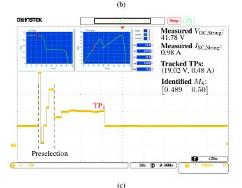
**FIGURE 8.** The tracked voltage traces recorded by the oscilloscope when searching the turning points for a PV string with four PV modules under (a) shading pattern 1: {1000,600,400,200}W/m², 25°C; (b) shading pattern 2: {800,500,1000,1000}W/m², 25°C and (c) shading pattern 3: {800,800,400,400}W/m², 25°C.
