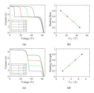
**FIGURE 5.** Relationships between the shading information and the position of the turning point for a PV string with five PV modules. (a) I-V curves with different shading rate information; (b) the relationship between the shading rate information and the voltage at the turning point  $V_{\mathrm{TP}}$ ; (c) I-V curves with different shading strength information; (d) the relationship between the shading strength information and the current at the turning point  $I_{\mathrm{TP}}$ .
