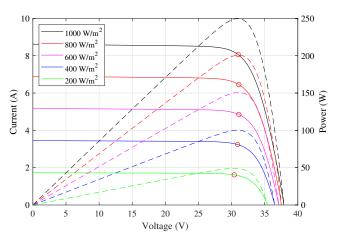
**FIGURE 1.** Electrical characteristics of a PV string under uniform irradiation conditions (UIC).
