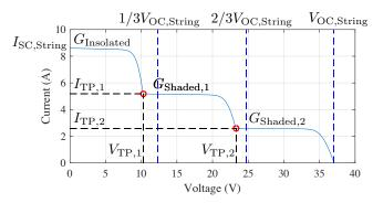
**FIGURE 2.** I-V characteristics of a PV string under partial shading conditions (PSC).
