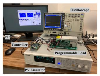
FIGURE 7. Experimental setup.
