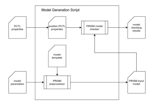
Figure 3.3: The automation of model generation and analysis for ant-based swarming models, given a set of parameters for the model and a set of PCTL properties to check.
