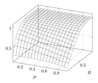
Figure 7.3: Parametric analysis of the crowds protocol for N = 5 internet users and R = 7 path reformulates. P is the probability that a user is untrustworthy, and B is the probability that a user sends a packet to a randomly selected receiver. The property of interest is the probability that untrustworthy users observe the sender more than they observe others.
