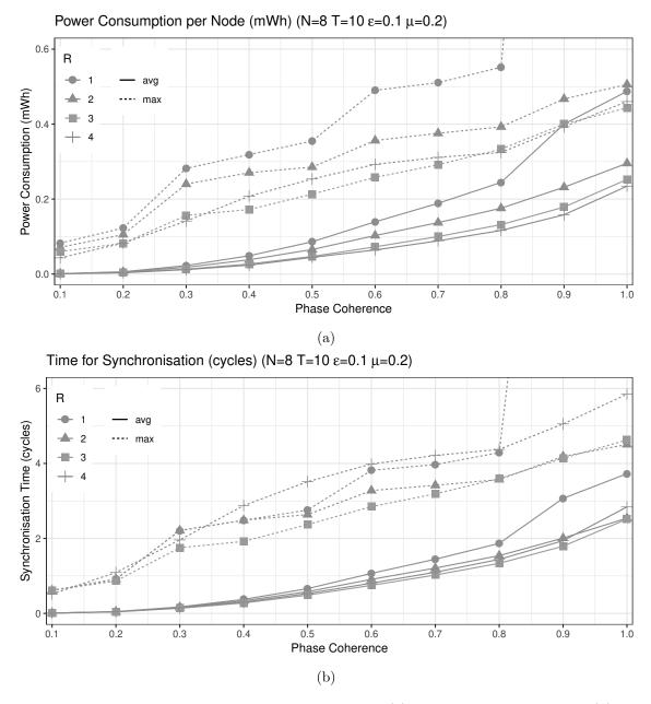
Figure 5.4: Expected rewards for power consumption (a) and synchronisation time (b) for a network of 8 nodes to achieve different degrees of phase coherence.
