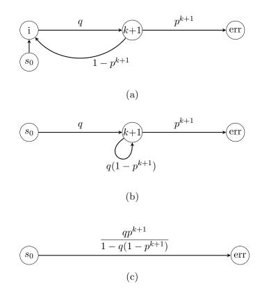
Figure 6.3:  $Z_{k+1}$  after the elimination of states k (a), i (b), and k+1 (c).
