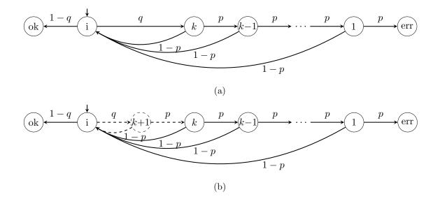
Figure 6.1: The zeroconf protocol for n = k (a) and n = k + 1 (b), where n is the number of attempts to check if the selected IP address is already in use.
