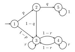
Figure 2.2: An example of a parametric Markov chain.
