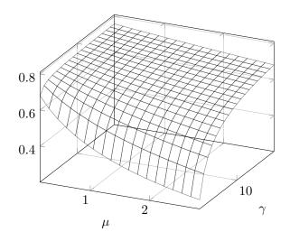
Figure 7.5: Parametric analysis of the cyclic polling server model for N = 4 clients.  $\mu$  is the service rate and  $\gamma$  is the rate at which the token is moved. The property of interest is the probability that, in the long run, a station is idle.
