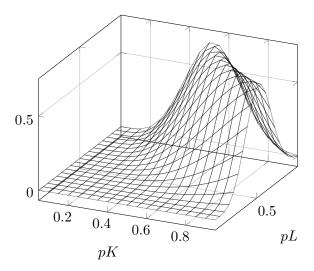
Figure 7.4: Parametric analysis of the bounded retransmission protocol for N = 256 file chunks and MAX = 2 maximum retransmissions over two lossy channels. The parameters pK and pL are the reliability of the data and acknowledgement channels, respectively. The property of interest is the probability that the sender reports an unsuccessful transmission after more than 8 chunks have been sent successfully.
