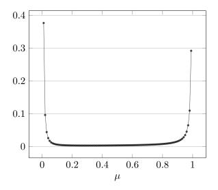
Figure 7.6: Parametric analysis of the oscillator synchronisation model for N = 6 nodes and T = 8 clock values. The parameter  $\mu$  is the probability of synchronisation messages being lost in the communication medium. The property of interest is the expected power consumption of the network (in Watt-hours) to reach a state, where the clocks of all nodes are synchronised.
