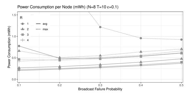
Figure 5.5: The relationship between broadcast failure probability and power consumption.
