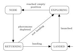
Figure 3.2: A finite state machine describing the behaviour of an MAV.
