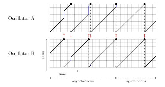
Figure 4.1: Synchronisation of two pulse-coupled oscillators.
