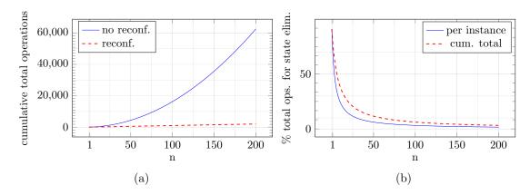
Figure 6.5: Cumulative total of arithmetic operations performed for iterative analysis of Zeroconf for n = 1...200 (a), and the per instance/cumulative ratios of total operations for reconfiguration to total operations for regular state elimination, given as a percentage (b).
