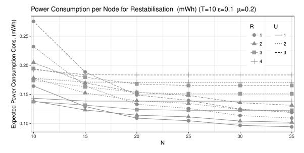
Figure 5.7: Power consumption for restabilisation for a range of network sizes.
