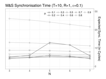
Figure 4.9: Synchronisation times for different number of oscillators for the Mirollo and Strogatz synchronisation model.
