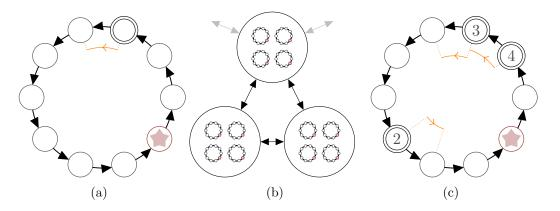
Figure 1.1: (a) A microscopic finite state automaton modelling the cyclic behaviour of an individual agent. (b) Three states of the composite automaton obtained by taking the product of individual microscopic models for four interacting agents. (c) A single state of the macroscopic model of four interacting agents, where counters are used to record agents sharing the same state.
