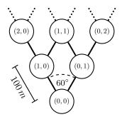
Figure 3.1: The Y-junction grid illustrating the ideal positions for MAVs. Each node is 100 m distant from each of its neighbours.
