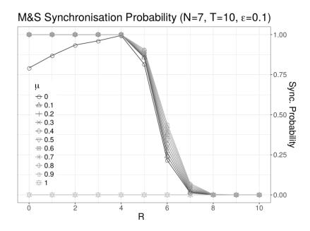
Figure 4.5: Mirollo and Strogatz synchronisation: synchronisation probabilities for different refractory periods.
