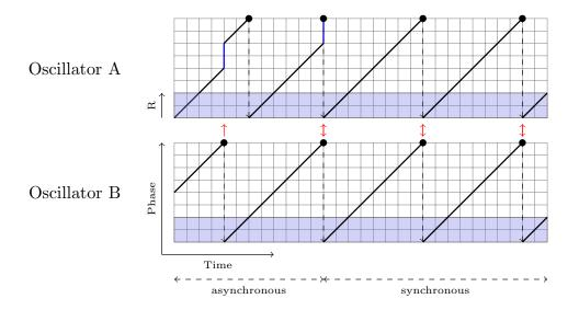
Figure 4.2: Synchronisation of two pulse-coupled oscillators with refractory periods.
