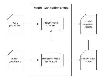
Figure 4.4: The automation of model generation and analysis for synchronisation models, given value ranges for model parameters, and a set of PCTL properties to check.
