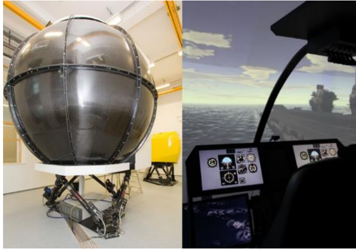
Fig. 2 QEC visual environment in the HELIFLIGHT-R flight simulator.
