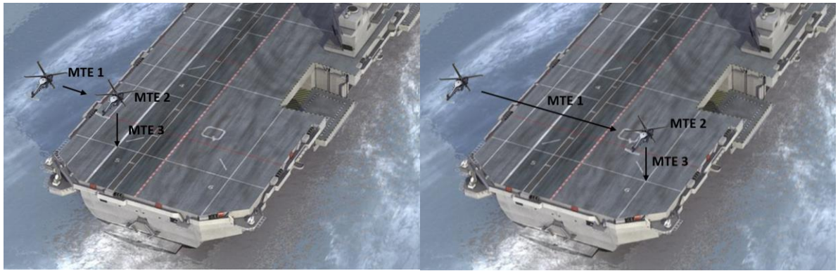
Fig. 8 Mission task elements on recovery to QEC landing spots 5 (left) and 6 (right).
