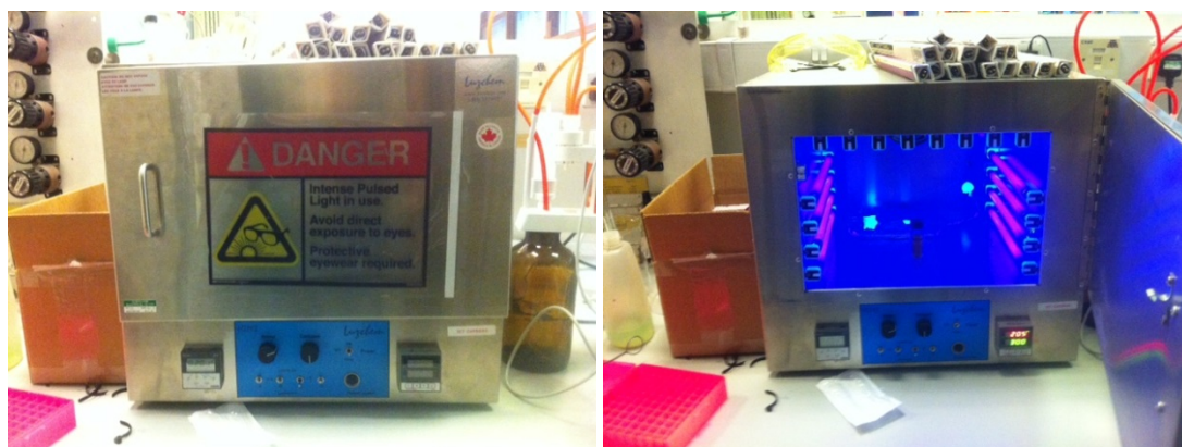
Figure 2.1 Photoreactor LuzChem ICH2. (16 UVA and 16 VIS lamps, 110 VAC, 50/60 Hz cycle, 4 Amps.)
