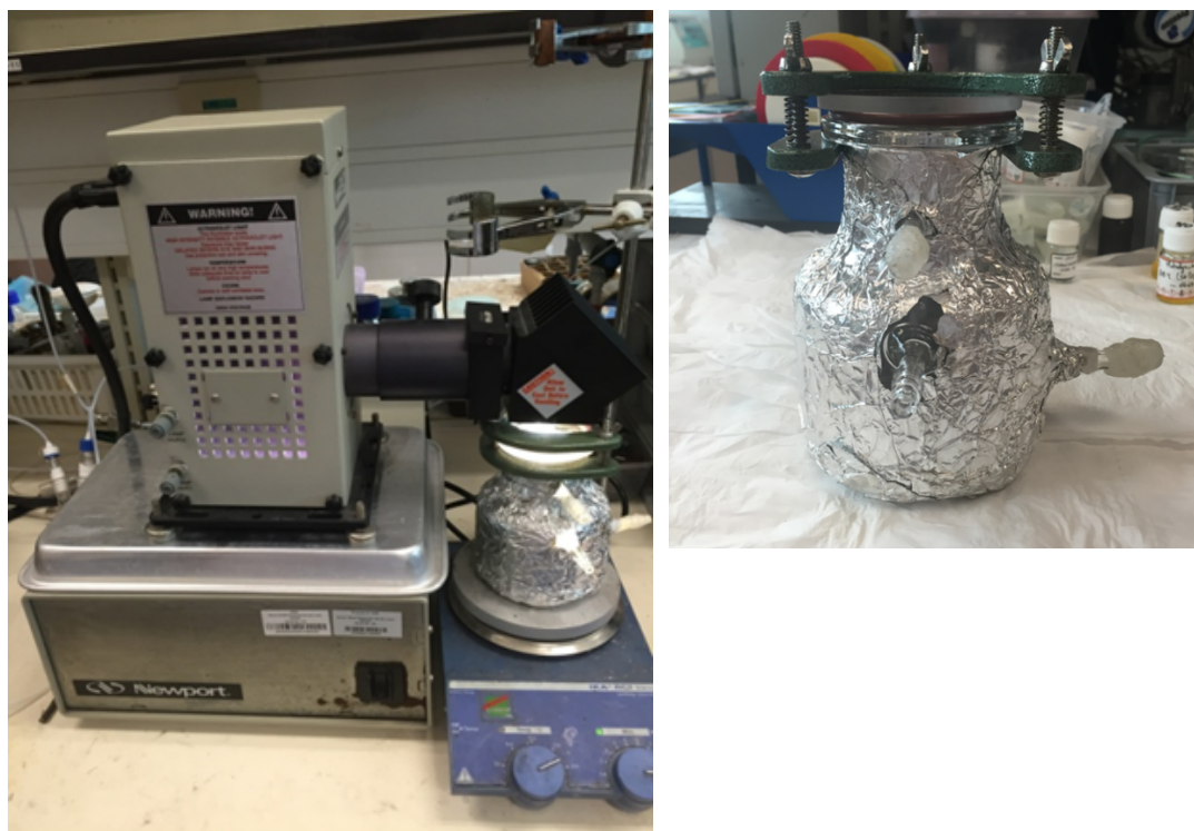
Figure 2.2. (Left) Photoreactor set up with 50 - 200 W research Arc Lamp Sources (Hg), produce collimated or focused output. (Right) photoreactor used in experiments for sonication-assisted nanoparticles.
