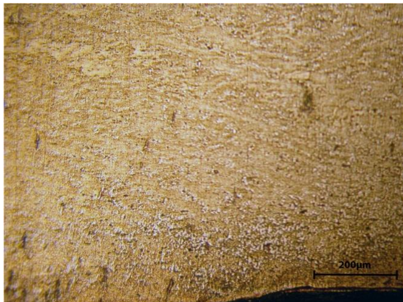
Figure 2. Photomicrograph of a section taken from a denarius of Otho (94% silver) showing deformed dendritic structure indicative of casting and cold-striking.
