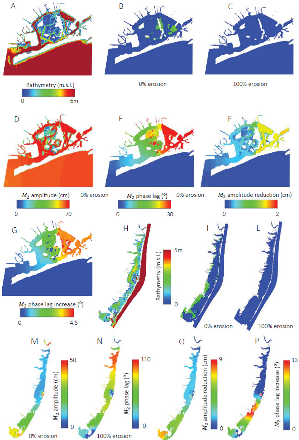
Figure A.4.2: bathymetry of Jamaica Bay and Barnegat Bay-Little Egg Harbor (a, h); model domains: current salt marsh distribution (b, i) and marsh completely eroded (c, l); M_2 amplitude (cm) and phase lag ( ^\circ ) for the 0% erosion case (d-e, m-n); reduction in M_2
