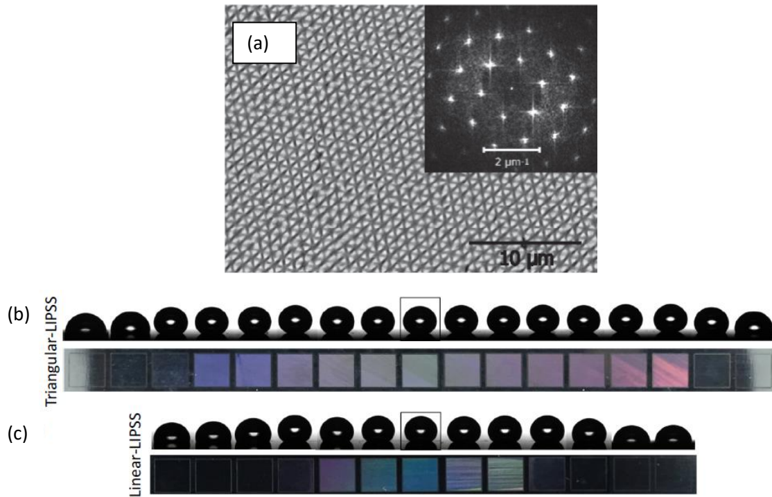
Figure 2. 19 Triangular-LIPSS produced by circular polarization. (a) Triangular-LIPSS pattern and corresponding Fast Fourier Transform (FFT). Bottom (b) Produced triangular-LIPSS for wettability properties modification (c) Produced linear-LIPSS for properties modification. [102].
