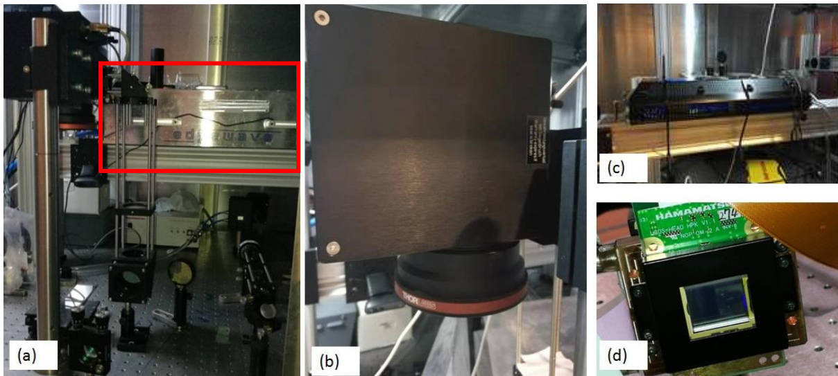
Figure 3. 7 Experimental device (a) A Edgewave laser indicated with a red rectangle (b) SCANLAB intelliSCAN 14 scan head with a F-theta lens, loaned from the University of Liverpool (c) SLM chiller (d) Hamamatsu X13138-03 SLM.
