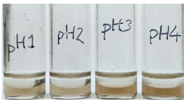
Figure 5. 15 – Photographs of the crown-AuNP solutions that have been left for 5 days. It can be seen that the decane phase is clear of crown-AuNPs
