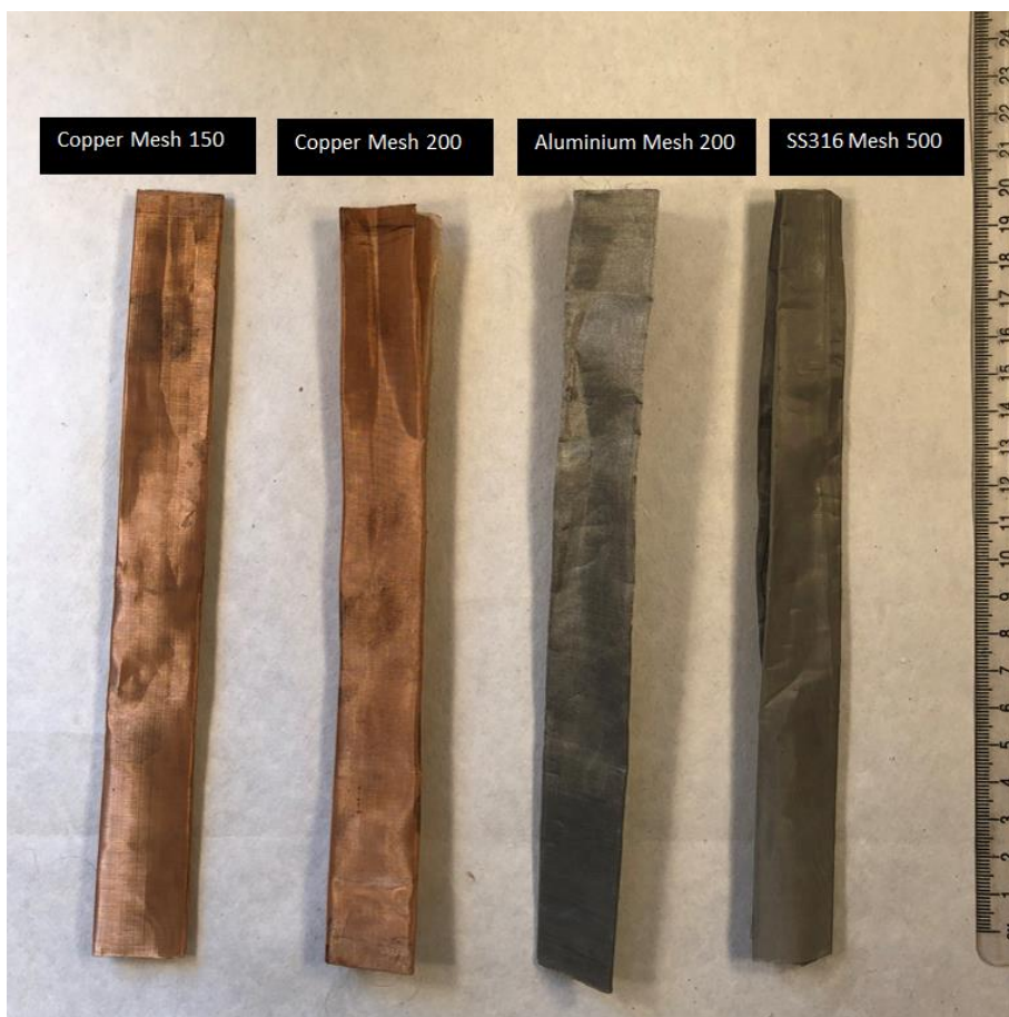
Figure 5- 14 Mesh wick samples with different mesh screens and materials
