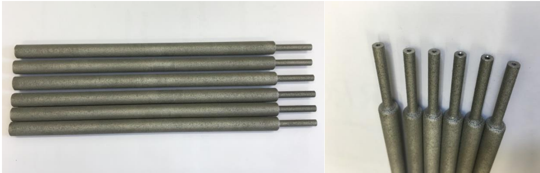
Figure 6- 4 As manufactured full length heat pipes with fill tubes and drilling holes
