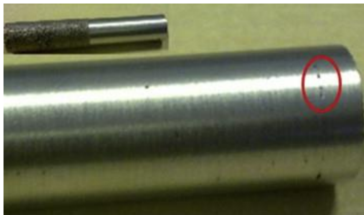
Figure 2- 19 Pores in an SLM solid structure (Ameli et al., 2013)
