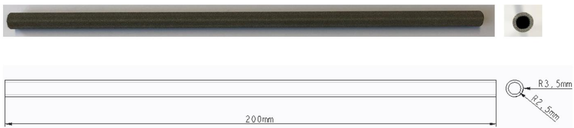
Figure 3- 14 Drawing of the porous tube made for capillary force testing
