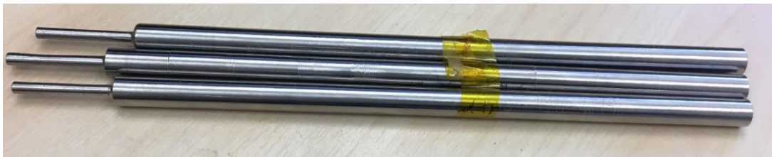
Figure 6- 5 Polished full length heat pipes
