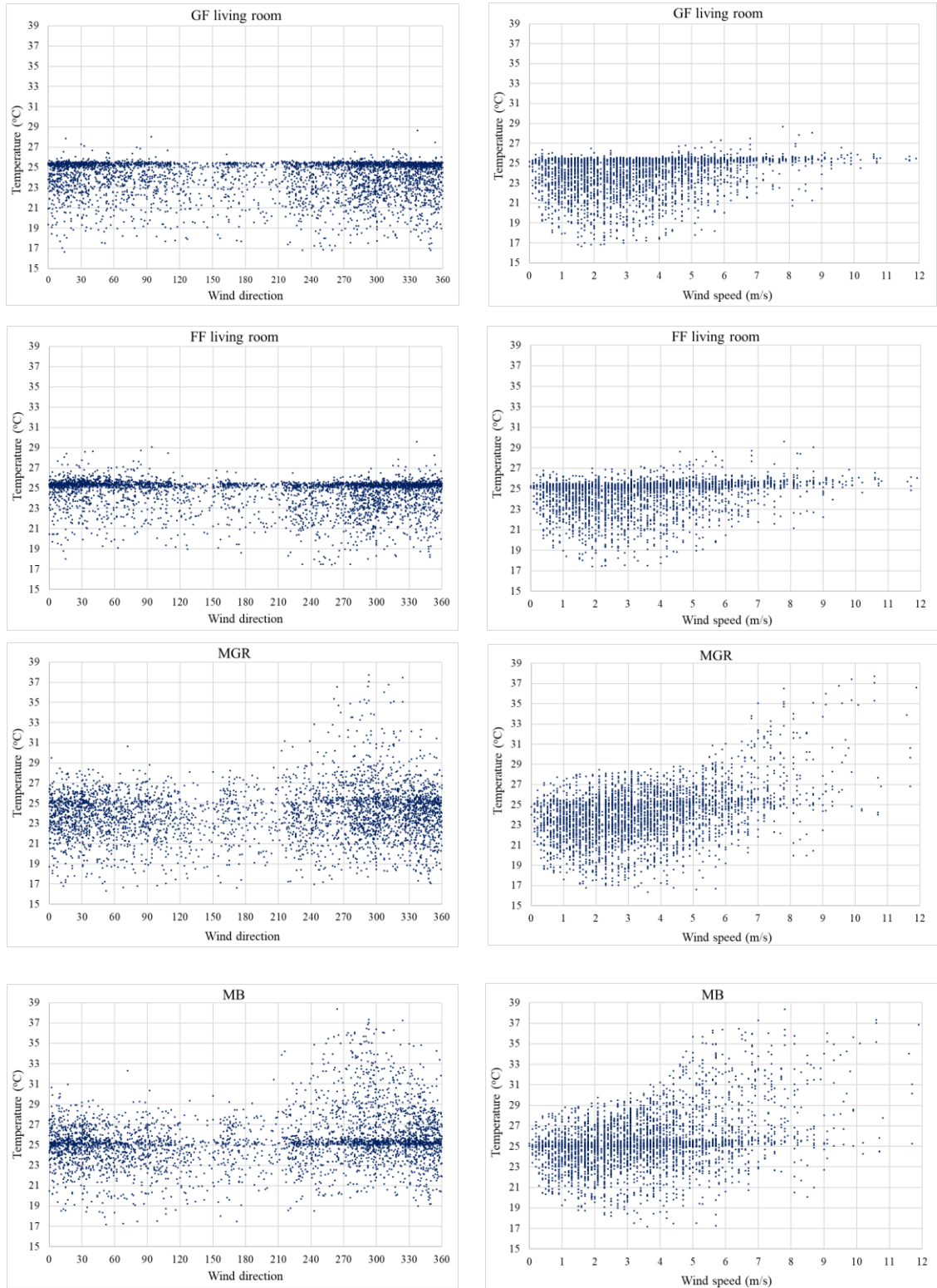
Figure 7-26: Wind direction effect (left) and wind speed effect (Right) on the four spaces during mixed-mode cooling
