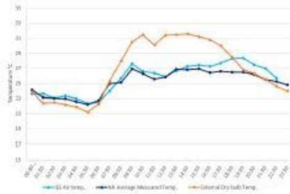
Figure 5: Comparison between measured and predicted internal air temperatures in room in Catania PDEC tower
