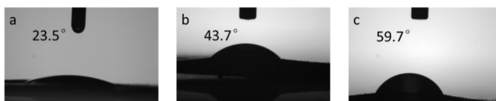
Figure 2-16. Water contact angles for pressed pellets of (a) FS-COF , (b) S-COF and (c) TP-COF at room temperature in air.
