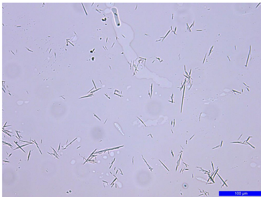
Figure 4.4- Optical microscope images showing the presence of SN-38 crystals in the aqueous phase.
