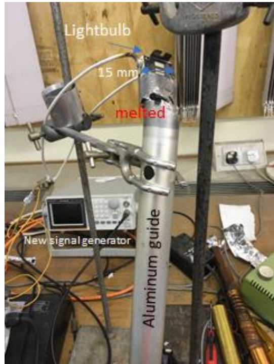
Figure 3-21 650W lightbulb heated the sample above 500 °C, but also heated the tube (locally) above 660 °C.
