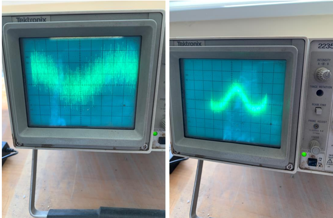
Figure 4-4 Tuning curves for two-axis computer-controlled system's gradiometer (left) and magnetometer (right). The scale is 0.5V; only the relative amplitude of the curves is relevant to the tuning process.
