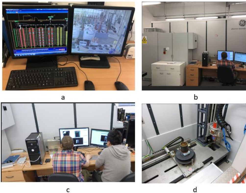
Figure 3.3. The v|tome|x L (modified) X-ray CT system. (a) The monitor; (b) the outlook; (c) the control panel; (d) manipulator in the chamber on which the sample is mounted.
