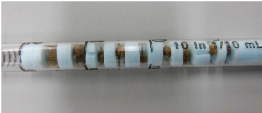
Figure 4.2. The aggregates were packed into a plastic tube to be scanned in the CT scanner.
