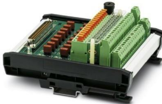
Figure 15 Custom Connection Interface for a PLC
