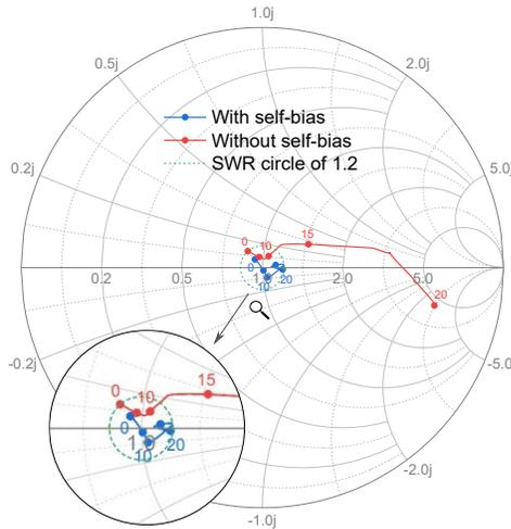
Fig. 6. The input impedance of the proposed rectifier in the Smith chart as a function of the input power with a sweeping range of 0 dBm to 20 dBm (1 dBm steps).
