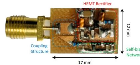
Fig. 9. Layout and photograph of the proposed rectifier.
