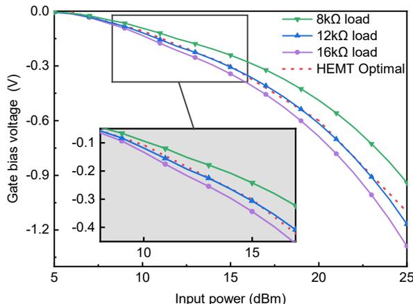
Fig. 5. The output voltage of the self-bias network with different load values as a function of the input power in measurement, compared with the optimal bias voltage for the HEMT obtained from simulation. The load value of the self-bias network can be chosen so that the network can always generate the optimal voltage for the HEMT.
