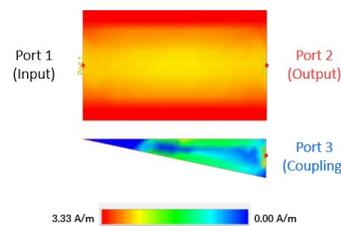
Fig. 3. Current distribution on the proposed coupling structure.
