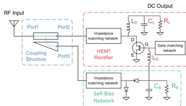
Fig. 1. Block diagram of the proposed rectifier.
