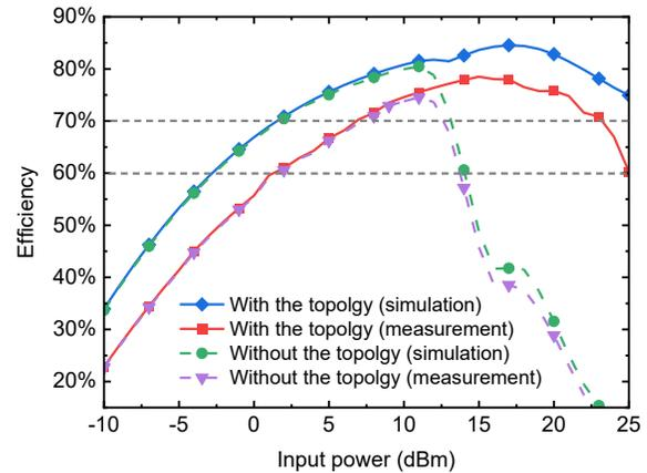
Fig. 8. The RF-DC conversion efficiency versus input power of the proposed rectifier with or with out the added self-bias network.
