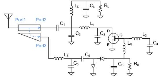
Fig. 7. Schematic of the proposed rectifier.
