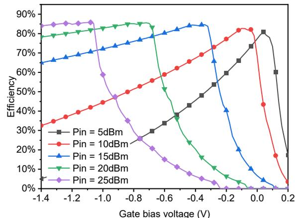
Fig. 2. Performance of the HEMT rectifier with different gate bias voltages
