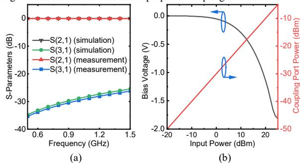
Fig. 4. (a) The S-parameters of the proposed coupling structure in simulation and measurement. (b) Bias voltage and coupling port power versus input power
