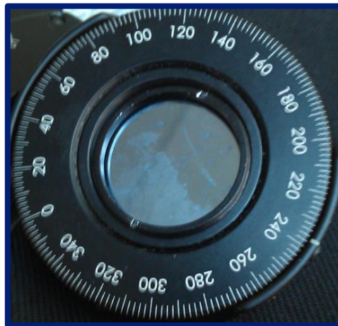
Figure 34: Image of a trimethoxypropylsilane (TMPS) functionalised silicon wafer adsorbed with human insulin (HI) and mounted in an optical rotation stage. The reflective silicon surface shows inhomogeneous insulin adsorption with blue colouration on differing aspects of the surface.
