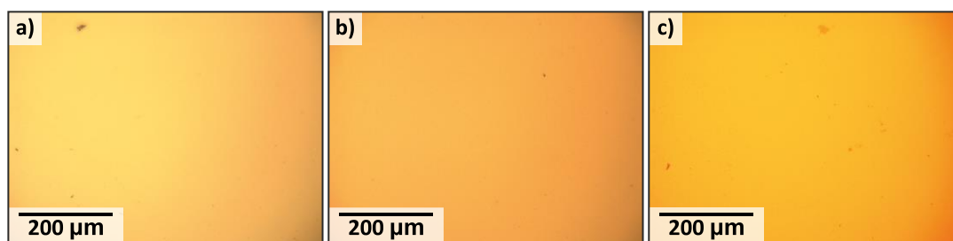
Figure 72: Optical microscopy images acquired at x20 magnification of the controls; (a) gold, (b) C 6 and (c) C 18 functionalised surfaces. No adsorbed species are observed in any of the optical images.
