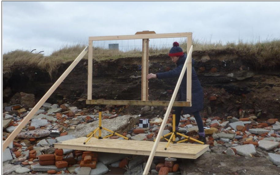
Figure 4.3: Camera grid at 'Height 1' on the levelled base - 2 m distance from frontage.
