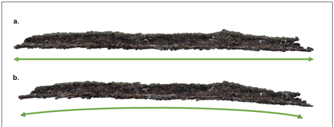
Figure 5.4: Crosby dense point cloud deformation under differing image alignment parameters. a) 'Medium' image alignment plus 'Ultra-High' densification. b) 'Highest' image alignment plus 'Ultra-High' densification.
