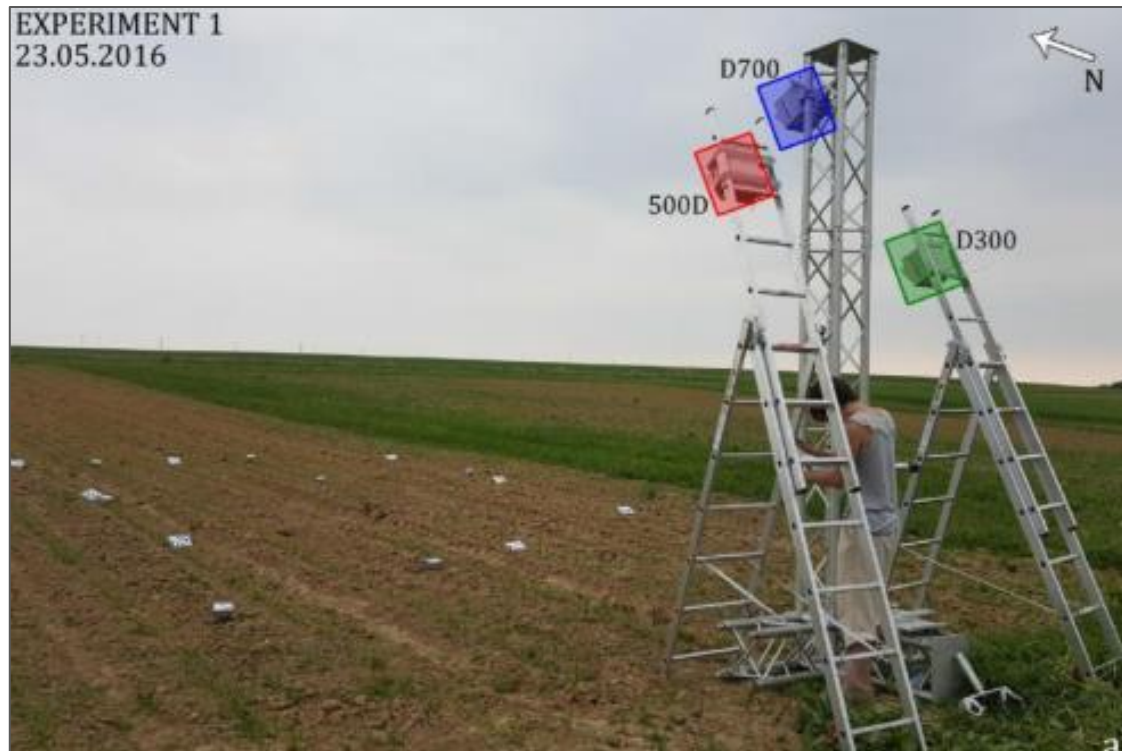
Figure 2.4: Image acquisition using three fixed cameras to monitor soil erosion after rainfall events. Source: Eltner et al. (2017).
