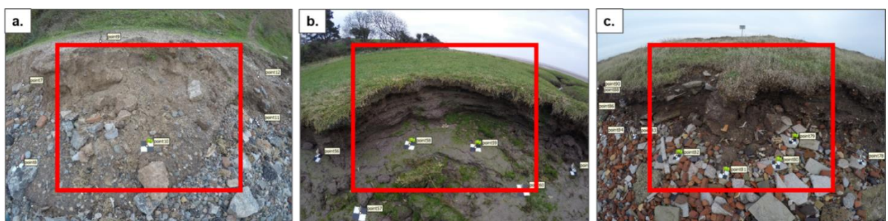
Figure 5.3: Example images used in the point cloud generation showing the estimated central placement of markers onto GCPs in Agisoft Photoscan a) Thurstaston b) Silverdale c) Crosby.
