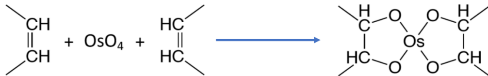
Fig. 2.13 Schematisation of osmium tetroxide reacting with unsaturated bonds in lipids. OsO 4 acts as a crosslinker and is reduced in the process. Image adapted from [24].
