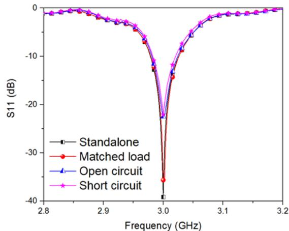
Fig. 15. Measured S11 of the Tx antenna when the Rx was connected to different loads.
