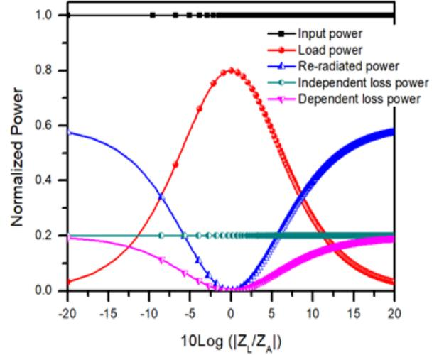
Fig. 9. The normalized various powers as a function of the impedance ratio of the load and antenna on a logarithmic scale for a lossy case.
