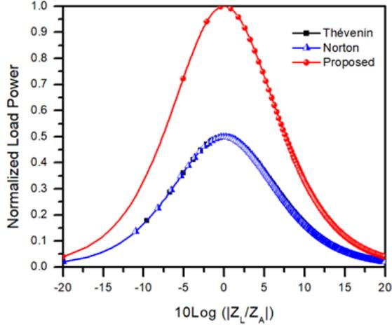
Fig. 8. The normalized load power as a function of the impedance ratio of the load and antenna on a logarithmic scale.
