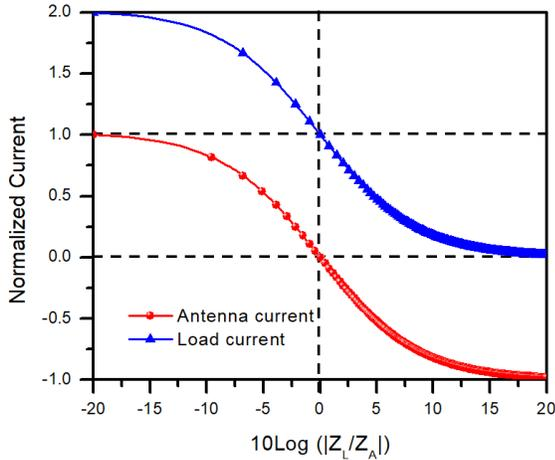
Fig. 11. The antenna current and the load current as a function of the impedance ratio of the load and antenna on a logarithmic scale
