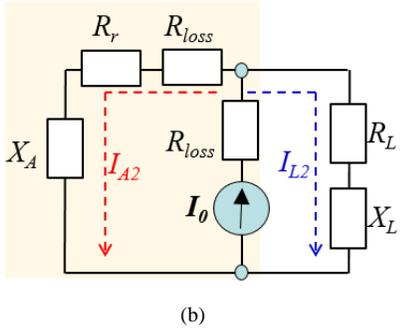
Fig. 7. Applying the superposition method to the proposed model by (a) replacing  $I_0$  with an OC (b) replacing  $V_0$  with an SC
