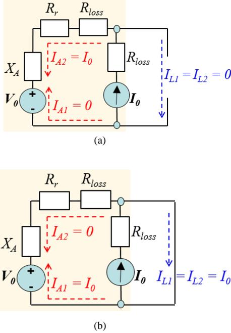
Fig. 10. The proposed receiving antenna model terminated by (a) an OC (b) an SC.
