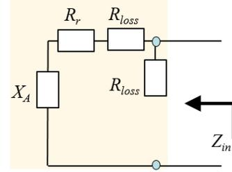
Fig. 12. The input impedance of the proposed antenna model using Thévenin theorem
