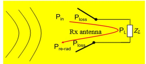
Fig. 5. The power going through a receiving antenna.
