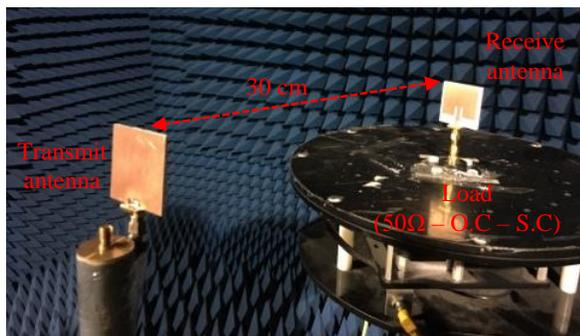
Fig. 14. Two patch antennas were used to measure the S11 with different loads.
