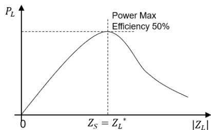
Fig. 2. The power at the load as a function of the magnitude of its impedance. At the peak, the power transfer efficiency is 50%
