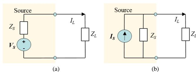
Fig. 1. The equivalent circuit of an antenna system: (a) The Thévenin equivalent circuit; (b) The Norton equivalent circuit.
