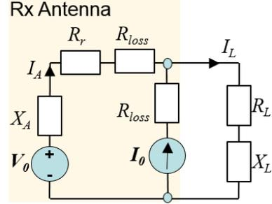
Fig. 6. The proposed receiving antenna model.
