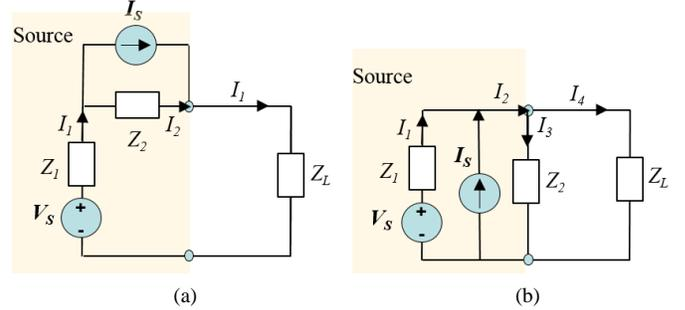
Fig. 3. Two constant power sources: (a) Series power source; (b) Parallel power source.
