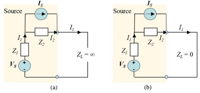
Fig. 4. The equivalent circuits of two special cases (a) an OC load (b) a SC load.
